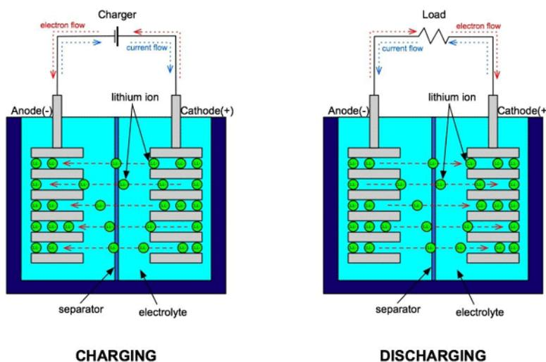
**Figure 29..** Charging and discharging process in Li-ion batteries [65]
