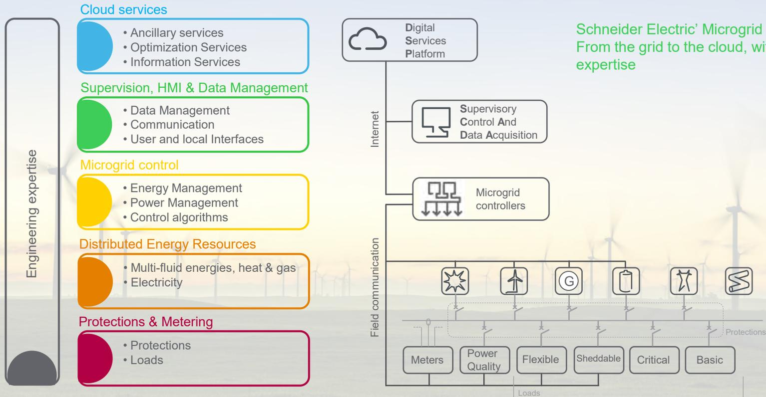
Schneider Electric' Microgrid architecture:
