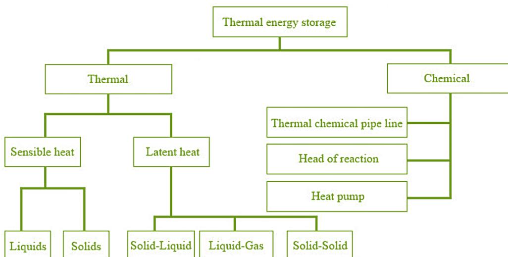
**Figure 13.** Types of solar thermal energy storage [24].
