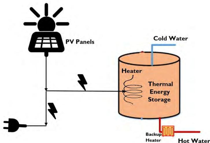
**Figure 14.** Typical schematic of a solar-thermal energy storage.
